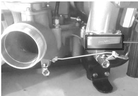
The pump serial (identification) number is marked on the pump casing.
